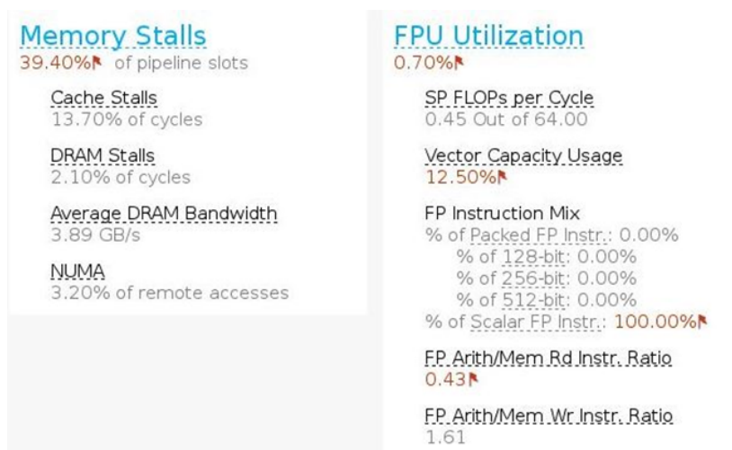
Figure 13 HemoCell Memory stalls and floating-Point Instruction usage – Intel Application Performance Snapshot
