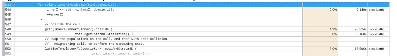
Figure 16 Palabos solver, blockwiseBulkCollideAndStream loop -- Intel VTune
