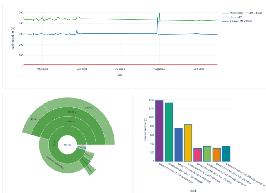
Figure 4. Other outputs produced by rooster, showing the evolution of the execution time for intel i4 vs the date, as well as the details of the duration of each code part, and a comparison with other builds.
